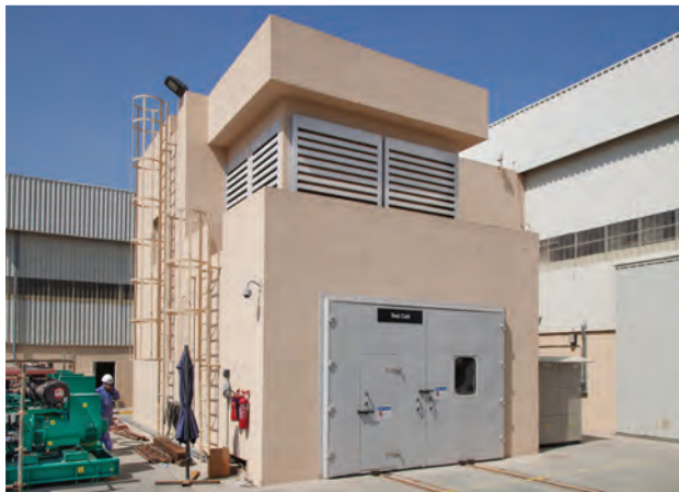
Genset Load test upto 2,500 KVA, 415V @pf 0.8 or 1.0
