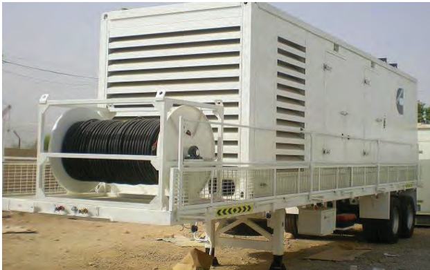
Mobile Power Pack. 1 MW supplied to RAECO. Multiple units were supplied. Each can parallel with utility or any other generator and run on Load Govern mode.
