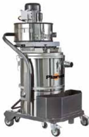
Brand: IPC SOTECO ATEX Model: Planet Optim 3m ATEX Wet & Dry Specifications Motor: 3 KW Air Flow (m3/h): 320 Waterlift (mm H2O): 3100 Filter Surfaces (cm2): 12000-24000 Tank Capacity: 50-70L Noise: dB(A)←85 Weight: 22 Kg
